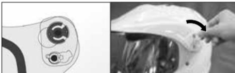
Pre-assemble the peak with screws, pressure plates and retaining plates making sure the slender part of the clip washer on each side points upward.
