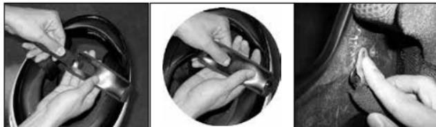
To replace the right chinstrap cover (long side), ensure the cap side of the chinstrap end snap (Arai logo impressed) on the chinstrap and the leatherette side of the chinstrap cover both face outward, slip the chinstrap cover onto the chinstrap.
