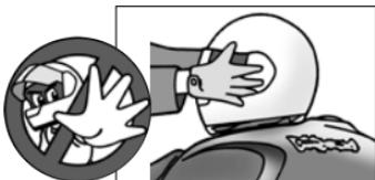
Do not expose helmets to solvents including gasoline, or their fumes to avoid damage to shields, small plastic components and interior.
