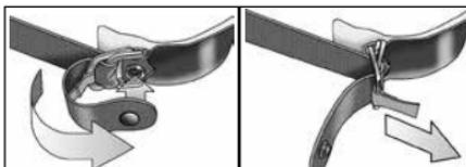
A D-ring release tab is provided to make loosening of the strap easier, simply pull as illustrated.
