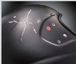
Right: Impact scars from drop test (hemisphere anvil) ▶
