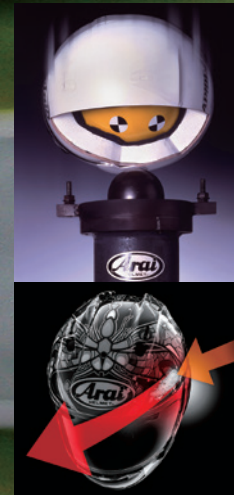
All helmets protect the rider's head through both glancing off and energy absorption.
