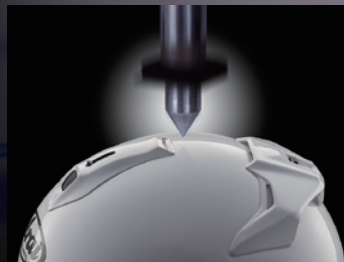
The helmet penetration test drops a 3kg striker onto the helmet from 3 meters up. The test confirms the strength of the helmet against failure from the road surface, obstacles in the road, footpegs, or other potential hazards.
